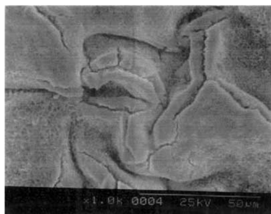
Figure 7 The top surface of type 2 specimen after 150 A cycles. More cracks seen than that of 75 A cycles.
