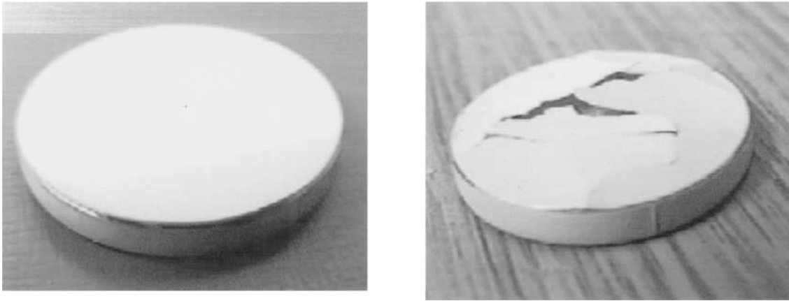
Figure 12 The spallation nature of type 1 specimen after 180 type A thermal cycles.
